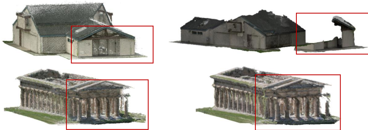
Figure 2. Examples of badly reconstructed dense clouds (drift effect) because of erroneously oriented images. Up: Barn_TaT dataset oriented with COLMAP -sequential (left) and AliceVision -SIFT-incremental (right). Bottom: Nettuno_aerial dataset, AliceVision + COLMAP (left), AliceVision + OpenMVS (right).
