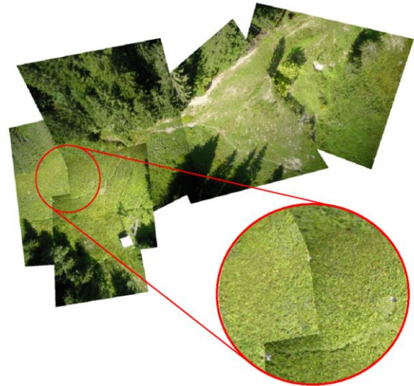
Figure 3. Mosaic of the Heumoes landslide with clearly visible image borders
