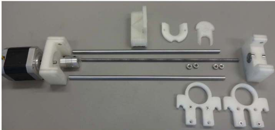
Figure 3. Exploded view of Open-Source Syringe Pump. doi:10.1371/journal.pone.0107216.g003
