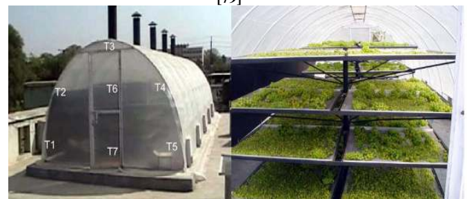
Figure 2.11 Hybrid photovoltaic-thermal (PV/T) integrated greenhouse dryer [79]
