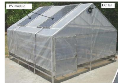
Figure 2.11 Hybrid photovoltaic-thermal (PV/T) integrated greenhouse dryer [79]
