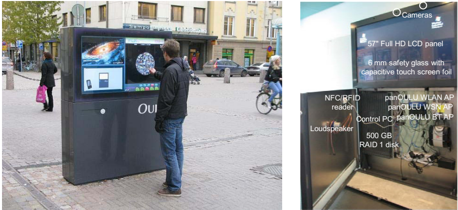
Fig. 3. (a) Outdoor UBI-display at downtown Oulu; (b) Components of an indoor UBI-display
