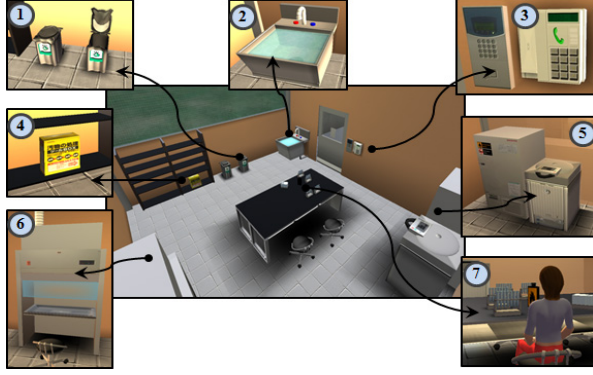
Fig. 2. OpenBioSafetyLab - Laboratory Appliances and Objects: (1) Waste bin, (2) Wash bin, (3) Intercom and Phone, (4) Fluid Spill Kit, (5) Fridge and Autoclave, (6) Biological Safety Cabinet, and (7) Experimental Table
