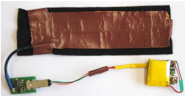
Figure 10. A wrist-worn accelerometer employing a proximity sensor with an invisible electrode in the wristband can enhance activity recognition by providing information about the object characteristics and their proximity [10].
