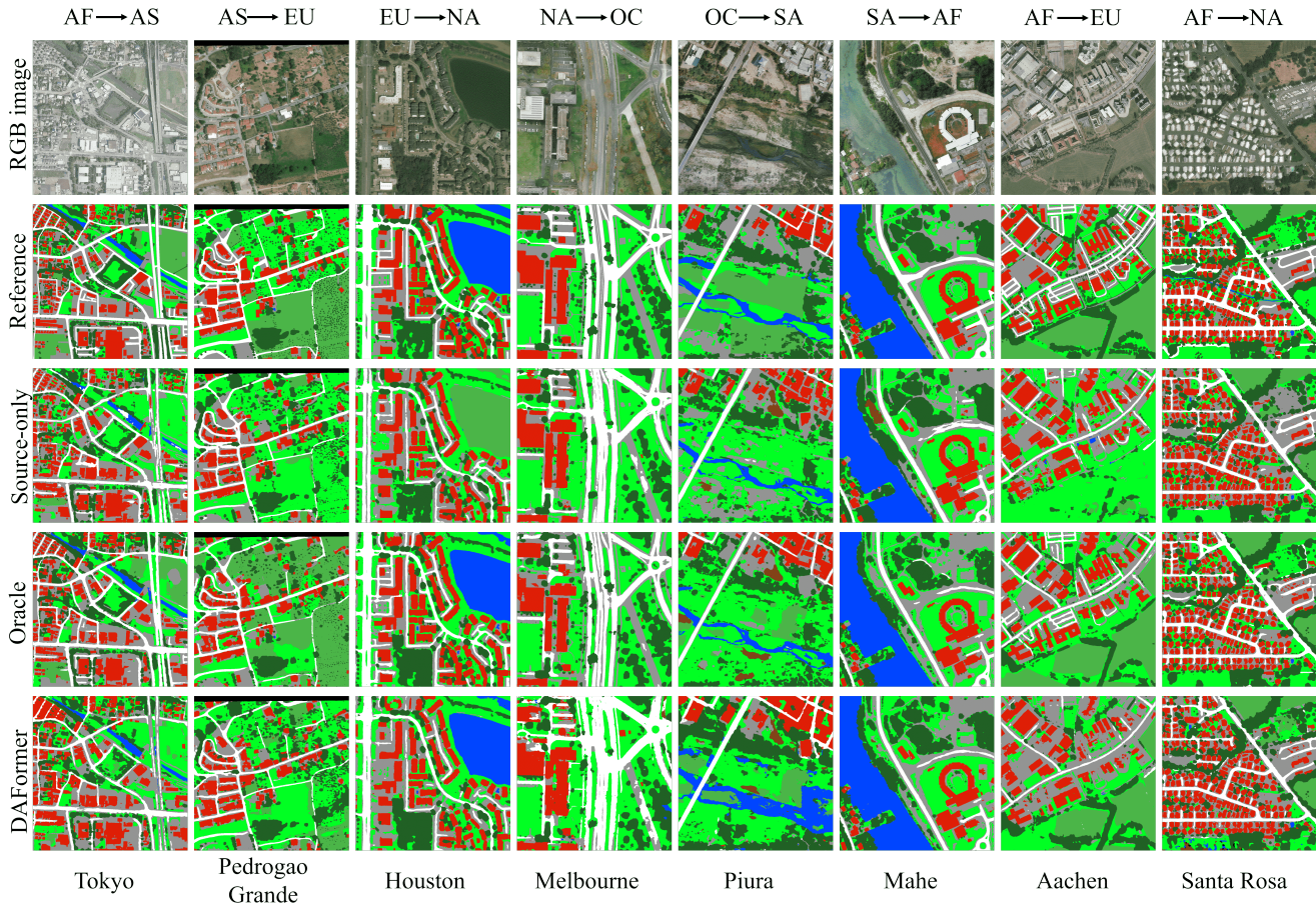
Figure S4: Visual comparison of continent-wise unsupervised domain adaptation results of source-only SegFormer, Oracle and DAFormer. Asia: AS, Europe: EU, Africa: AF, North America: NA, South America: SA and Oceania: OC.
