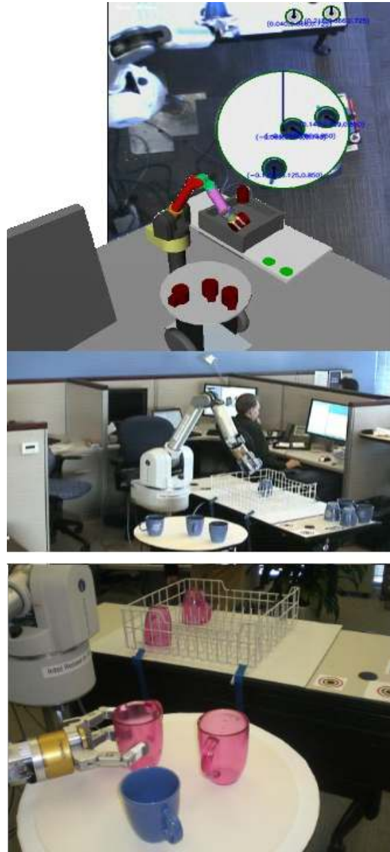
Figure 2: WAM loading cups from a segway to a dishwasher. OpenRAVE is used to sense and plan arm motions in real-time. An overhead camera ( top image ) tracks the segway, cups, and table, and feeds relative pose estimates to the OpenRAVE arm motion planning plugin.
