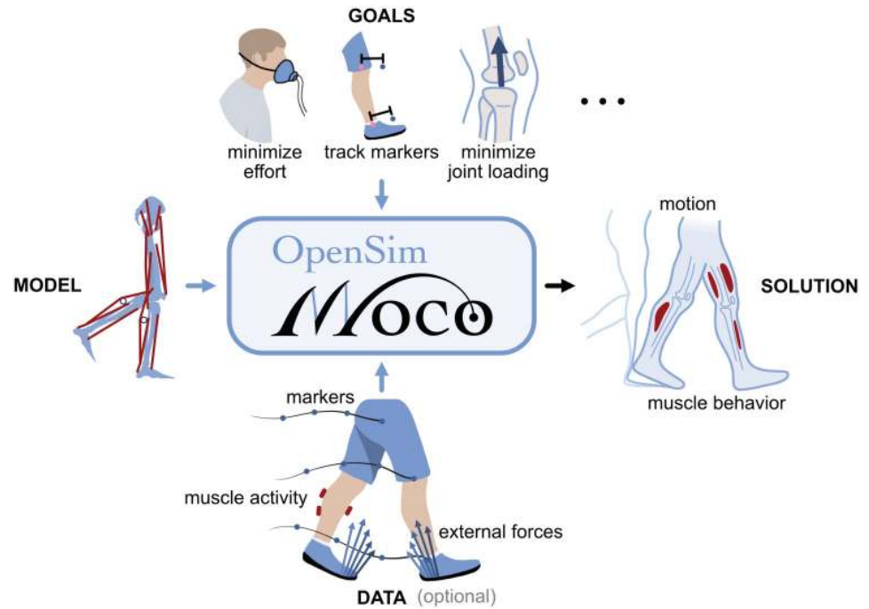
Fig 1. Overview of Moco. OpenSim Moco produces the optimal motion and muscle behavior for an OpenSim musculoskeletal model [54], given goals to achieve during the motion and reference data. Moco provides a library of goals, such as minimizing effort (illustrated with an indirect calorimetry mask), deviation from marker data (or generalized coordinate data), and joint loading. Reference data for the motion (markers or generalized coordinates), external forces (from force plates), and muscle activity (from electromyography) are optional. Illustration credit: Kai Rasmussen.
