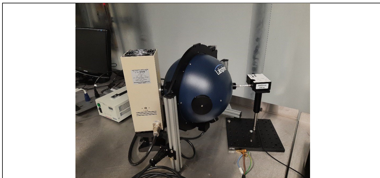
Figure 3-1. Large integrating sphere (10 inches in diameter) used to collect these measurements.
