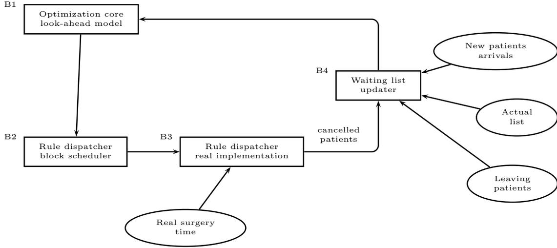
**Fig. 1** Structure of the optimization framework
