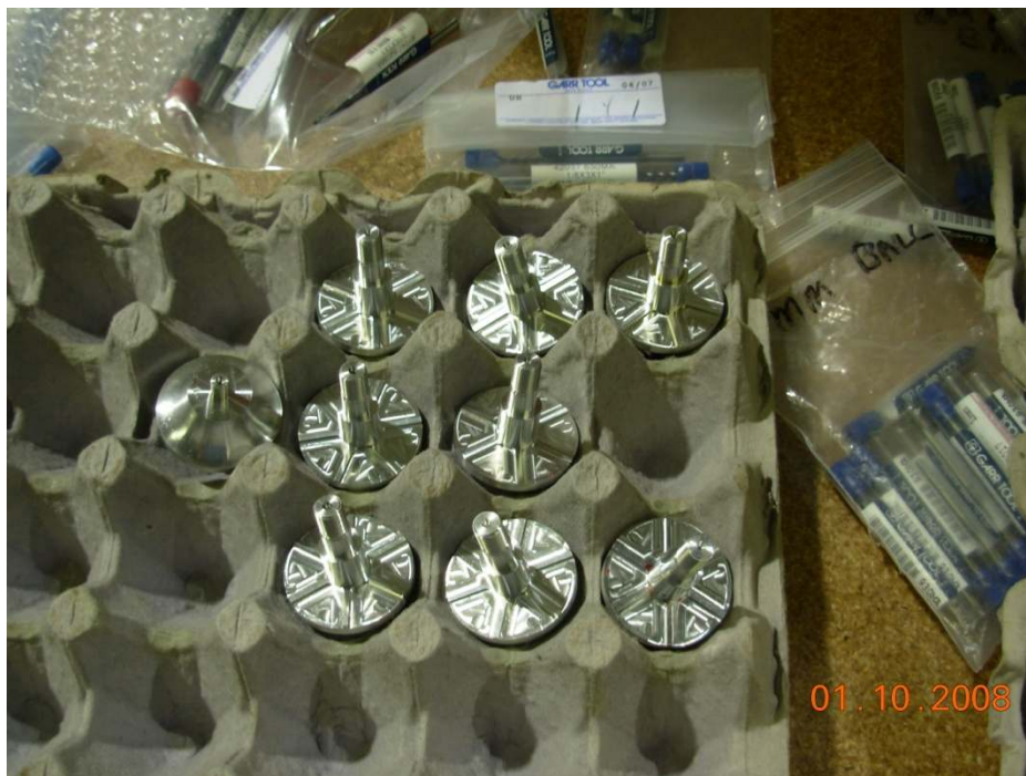
Figure 5-30: Multiple compressor wheels are provided to allow for several attempts to balance the thrust load. The pump-out vanes that are on the back of each wheel are shown. The height of the pump out vanes can be trimmed to reduce the load on the compressor wheel.
