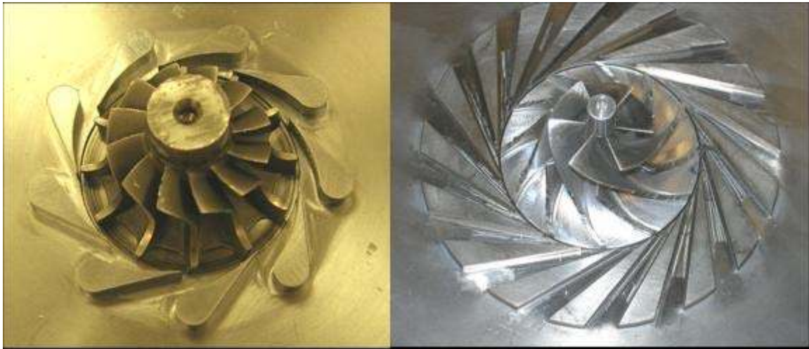
Figure 5-35: Photo of the 1.215" OD turbine and nozzle (left) and the 1.471" OD compressor with its diffuser (right).
