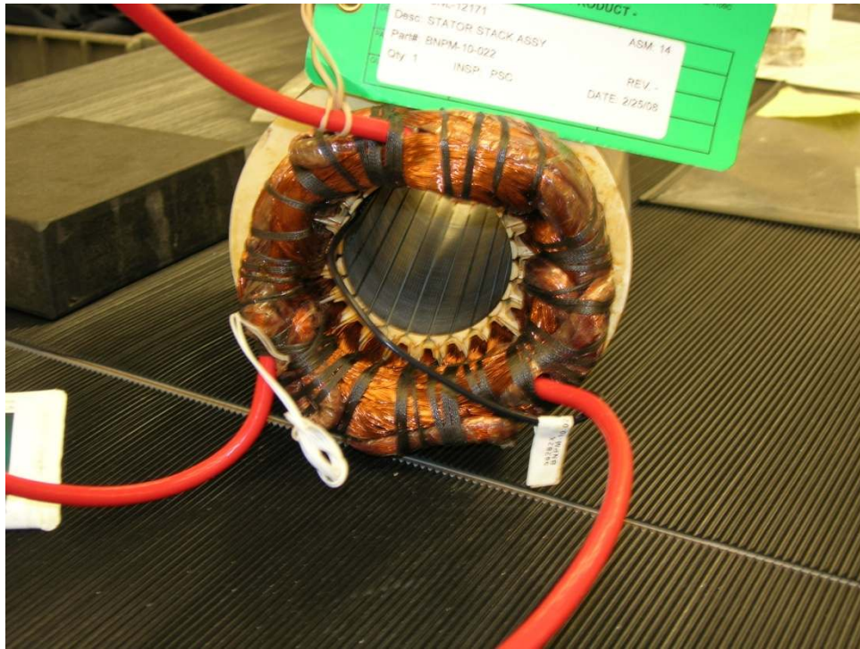
Figure 3-15: Photo of the PM stator for the supercritical CO 2 compression loop.
