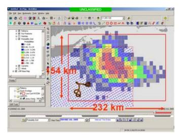
dicted dispersion of the 5000 simulated drifters using the HYCOM data source is shown in Figure 6. The search area using the HYCOM data equates to 36,000 km<sup>2</sup>. The predicted dispersion after 4 days of the 5000 simulated drifters using the HF radar data source is shown in Figure 7. The search area using the HF radar data equates to
