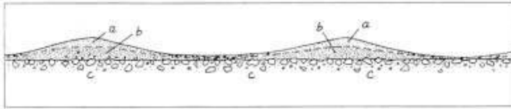
Figure 4.15 Schematic profile through a normally corrugated road surfaced with fine sandy aggregate (Beskow, 1932).
