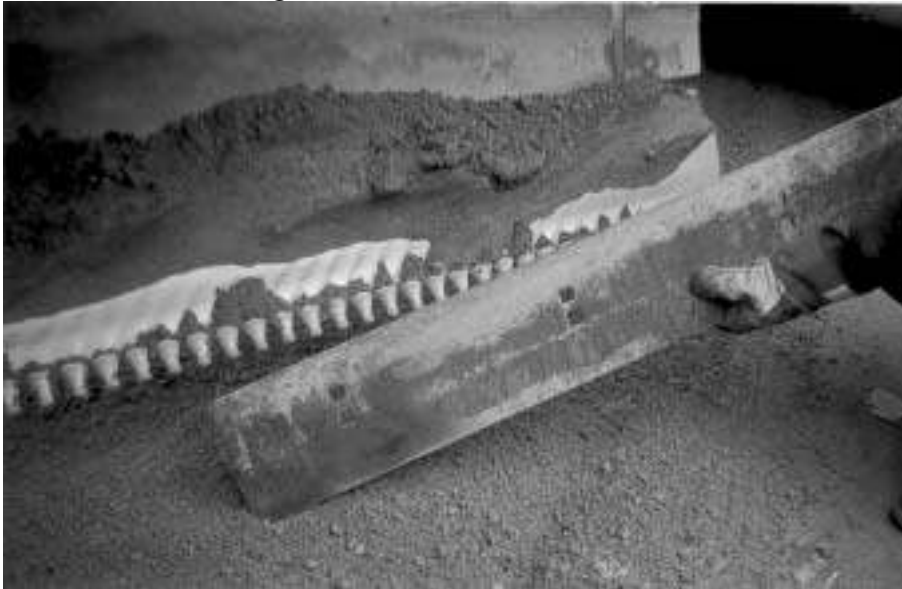
Figure 7.19 At front, smooth blade and behind, System 2000 that is mounted on the blade (Road maintenance-roads free from snow and ice, 1992).
