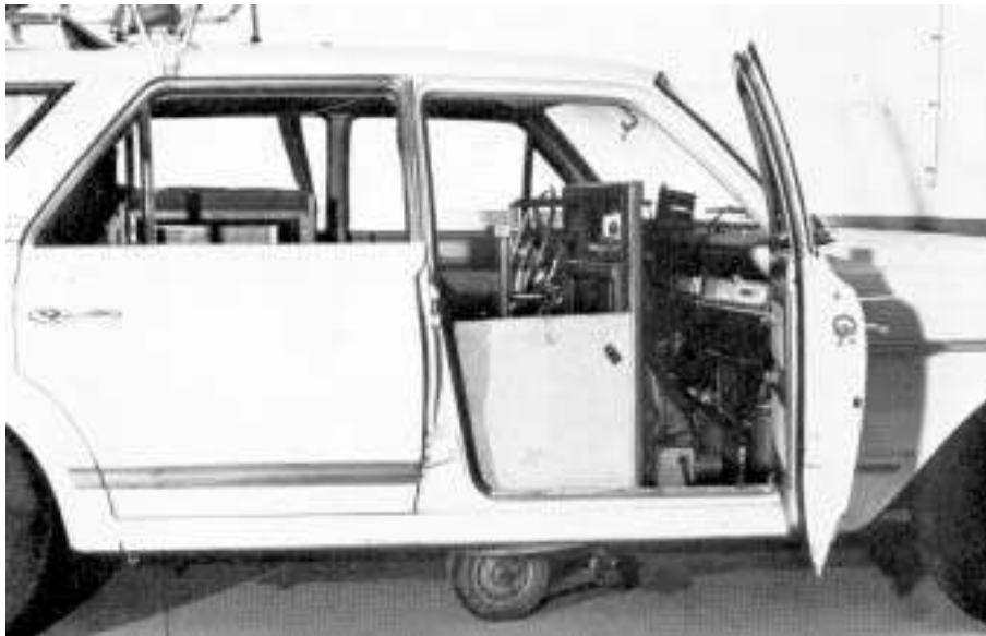
Figure 8.7 GM Profilometer (Magnusson et al., 1977).
