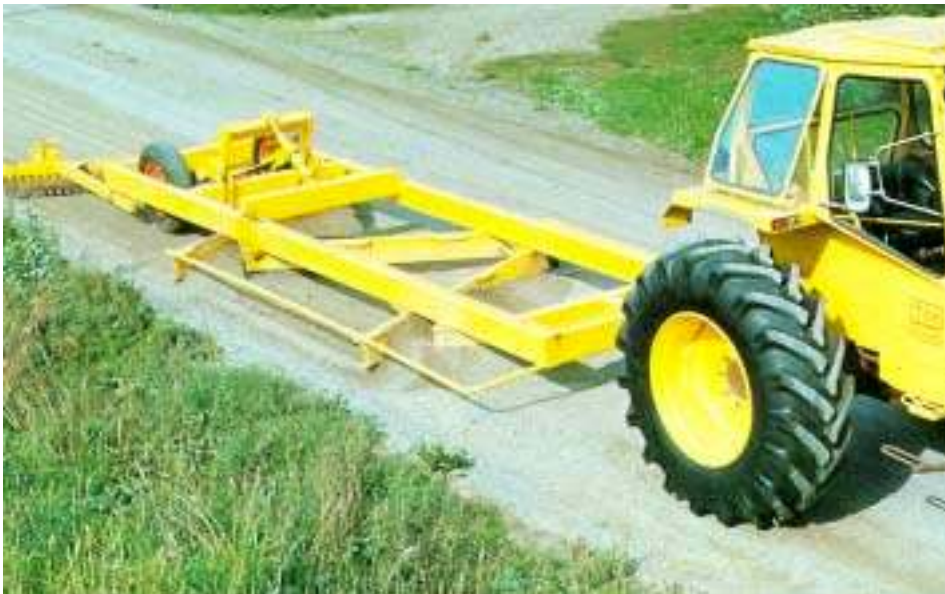
Figure 7.24 Road drag coupled to a tractor ( Maintenance of gravel and earth roads, 1994 ).
