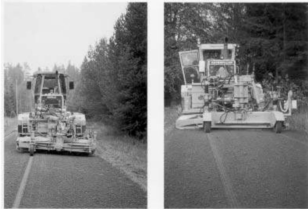
Figure 7.17 Windrow spreaders. At left, made by Mähler, and at right, made by Kommunalmaskin (Road maintenance-roads free from snow and ice, 1992).
