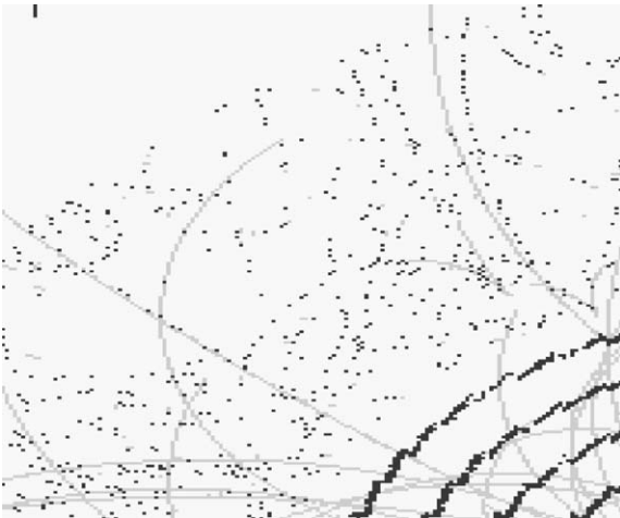
Fig. 10. The same as Fig. 9, after having applied the gate shown in Fig. 8 to minimise contribution from pile-up hits.
