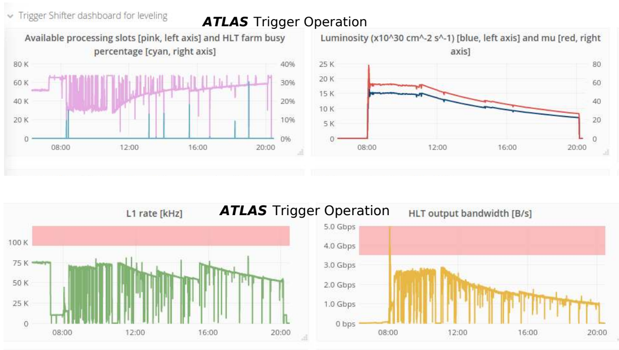
Figure 18: An example of a P-BEAST dashboard as used by the shifters during 2017 operation. The HLT farm availability (top left), the luminosity and the pile-up, ' \mu ' (top right), the total L1 accept rate (bottom left), and the total HLT output bandwidth (bottom right) are shown.
