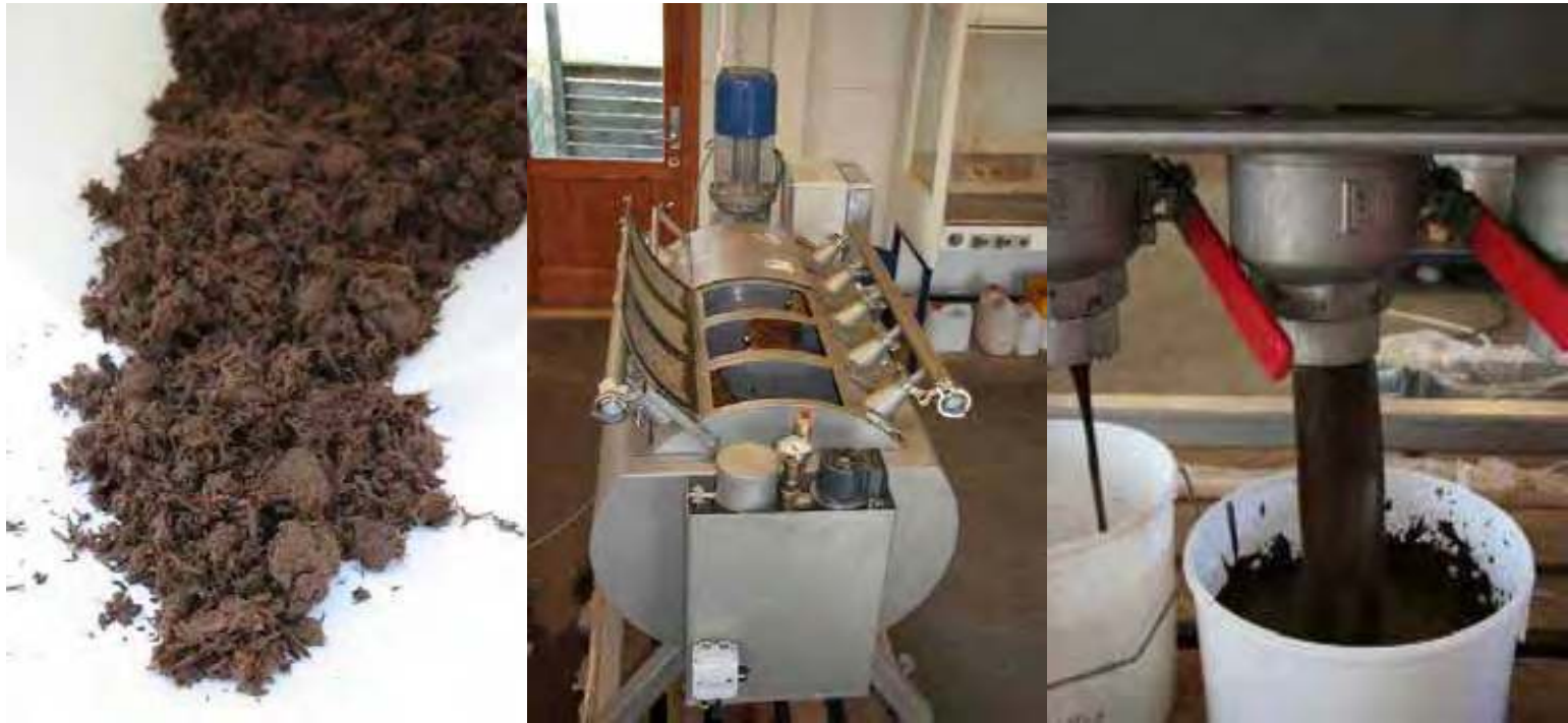
5 Chamber Liquifaction Reactor
