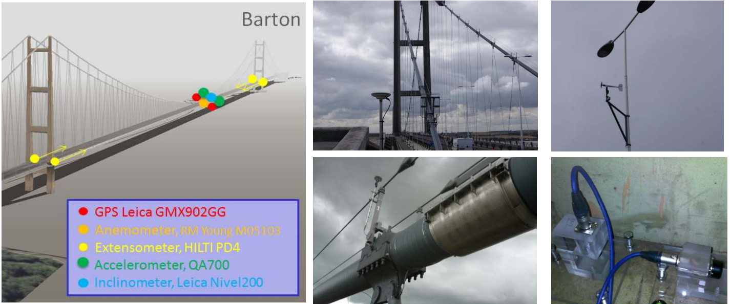
Figure 7: Humber Bridge (deformation) monitoring system and sensors: GPS antenna on anchorage and main cable; anemometer and accelerometers.
