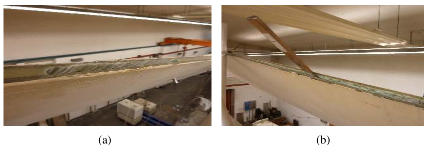
Figure 3 : Debonding introduced in the trailing edge of an SSP 34 m blade. (a) Original drilled debonding. (b) Extended debonding.
