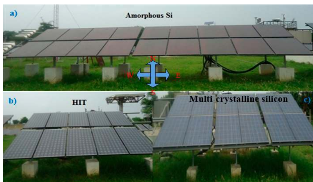
Figure 1. Experimental photovoltaic test facility at NISE, Gurgaon, India: (a). 1.2 kW Amorphous Si PV system; (b). 1.68 kW HIT PV system; (c). 1.6 kW Multi-crystalline silicon PV system.
