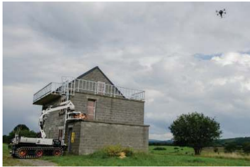
Figure 24. Large UGV deploying small UGV on the first floor, assisted by the outdoor rotorcraft (source: ICARUS).
