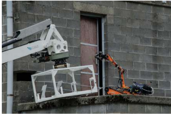
Figure 26. Small UGV opening a door with the manipulator arm, remotely operated by the exoskeleton (source: ICARUS).
