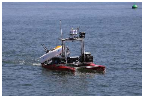
Figure 8. Unmanned capsule being launched from ROAZ II (source: ICARUS).
