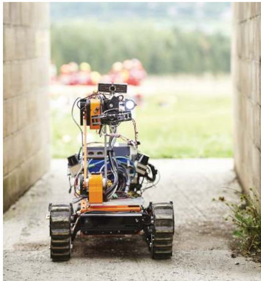
Figure 20. Unmanned ground vehicle navigating through the corridors of the building (source: ICARUS).
