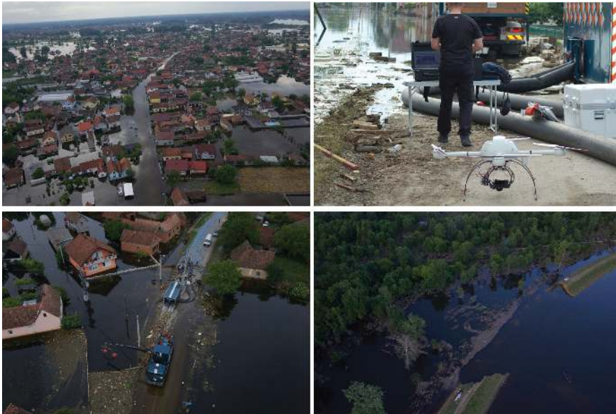
Figure 28. Top left: Flooded city of Orasje; top right: UAV used for the operations; bottom left: optimization of the location for the B-FAST water pumps and bottom right: broken dam on the Sava river detected by the UAV (source: ICARUS).
