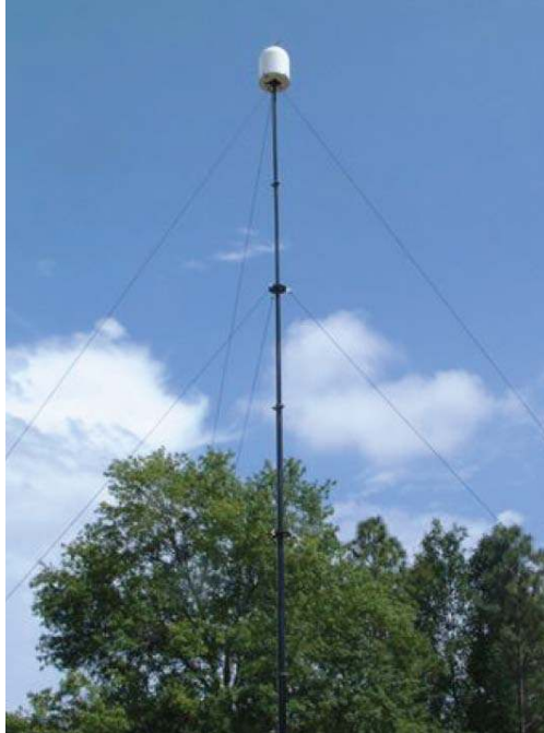
Figure 8. E600 Tactical Weather Radar Tower (EWR Weather Radar Systems 2006)
