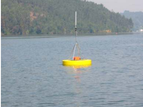
Fig. 1. Buoy with underwater acoustic beacon
