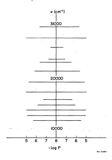
Fig. 1. A comparison between experimental and theoretical oscillator strengths of transitions in aqueous solutions of NdCl<sub>3</sub>. The lengths of the horizontal lines running from the central vertical line give a measure of -log P; theoretical values are given on the left, experimental values on the right. The ordinate of a horizontal line gives the approximate energy of the corresponding transition, in cm<sup>-1</sup>.
