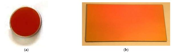
**Figure 3.** The general view of the optic filters with interference Si–SiO coating, formed on a sapphire substrate: (a)—a round sample with a diameter of 30 mm; and (b)—a rectangular sample with dimensions of  $150 \times 80$  mm.
