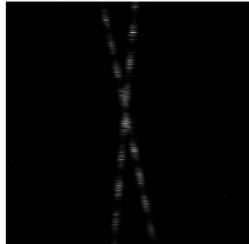
Figure 3. Single frame from a preliminary experiment to implement bandpass telescopy using a fibre-linked fringe transmission system. Note the speckle shown in the horizontal stripes within this data.
