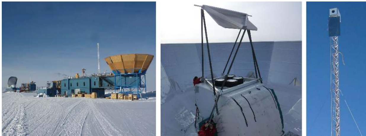
Figure 4: The setup for measuring far-field beam pattern of Keck Array detectors in situ at the South Pole. A chopped, broadband, microwave source broadcasts from a mast on the Dark Sector Laboratory (DSL), and a large aluminum honeycomb mirror is installed to redirect the beams of the Keck Array to the source. Left: The Keck Array in the foreground, with DSL in the background. Middle: The aluminum honeycomb mirror, installed on the Keck Array for beam measurements. Right: The microwave source mounted on a mast on the roof of DSL.
