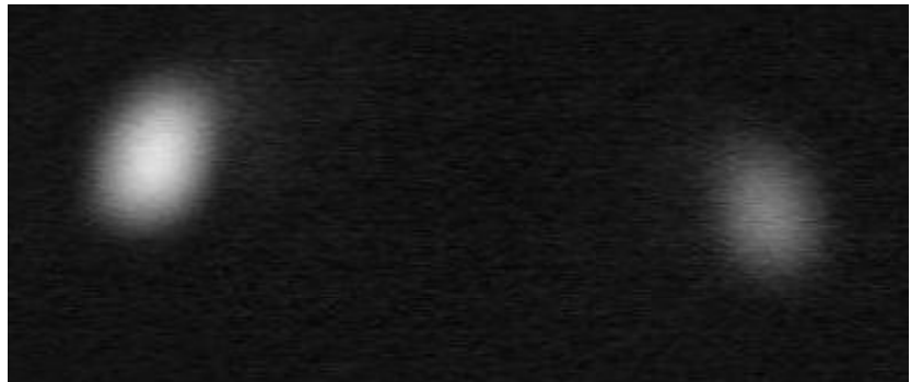
Figure 7. Sample image from the interferometer reference camera (CCD COH-REF). This separately shows each image (original and flipped) of a beam after having drilled through 50\ \mu\text{m} of aluminum. The slight asymmetry in the image of the hole emphasizes that one beam is a faithful mirror image of the other. The difference in intensities is a result of the glass plate in one beam.
