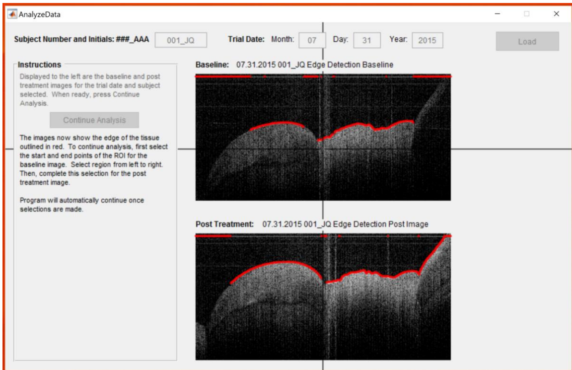
Figure 32 – MATLAB GUI for manual selection of region-of-interest for baseline and post-treatment options.
