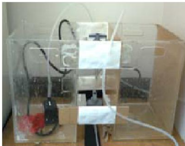
Fig. 5.3 (a) An illustration of the experimental setup of the cold block to activate/deactivate action potential propagation through the nerve while electrical recording is done at the end of the nerve (b) Implemented cold block. Two tanks to contain cold and hot solution(left) and two metallic tubes of the cold block(right) [108].
