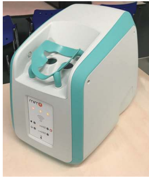
Fig. 6 Home-based MIMO-OCT system. Images courtesy of Dr Peter Maloca, University of Basel.
