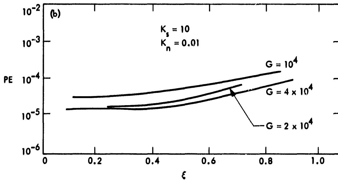
Figure A-1. PPM Error Probabilities in the Presence of Thermal Noise:
