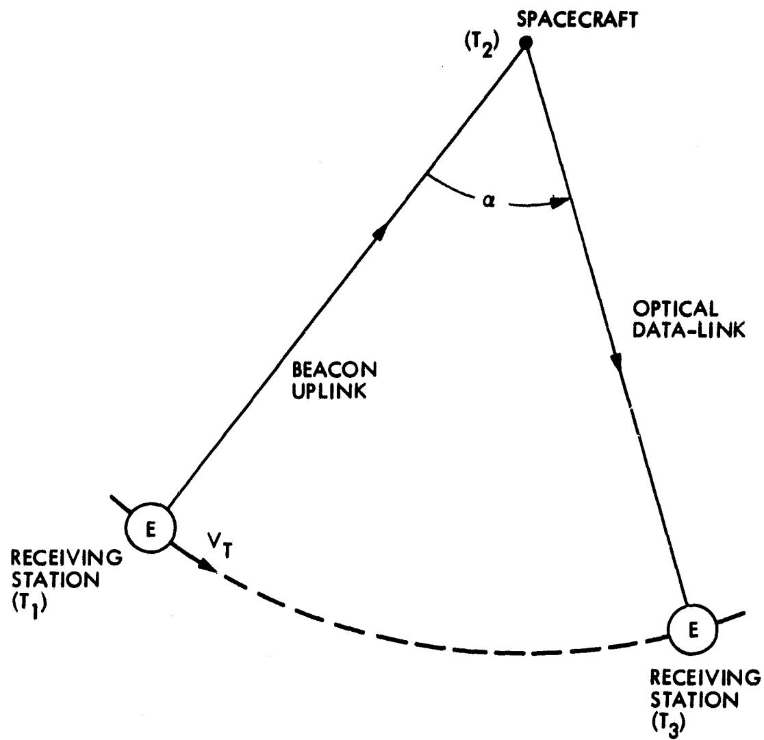
Figure 6-1. Point-Ahead Geometry
