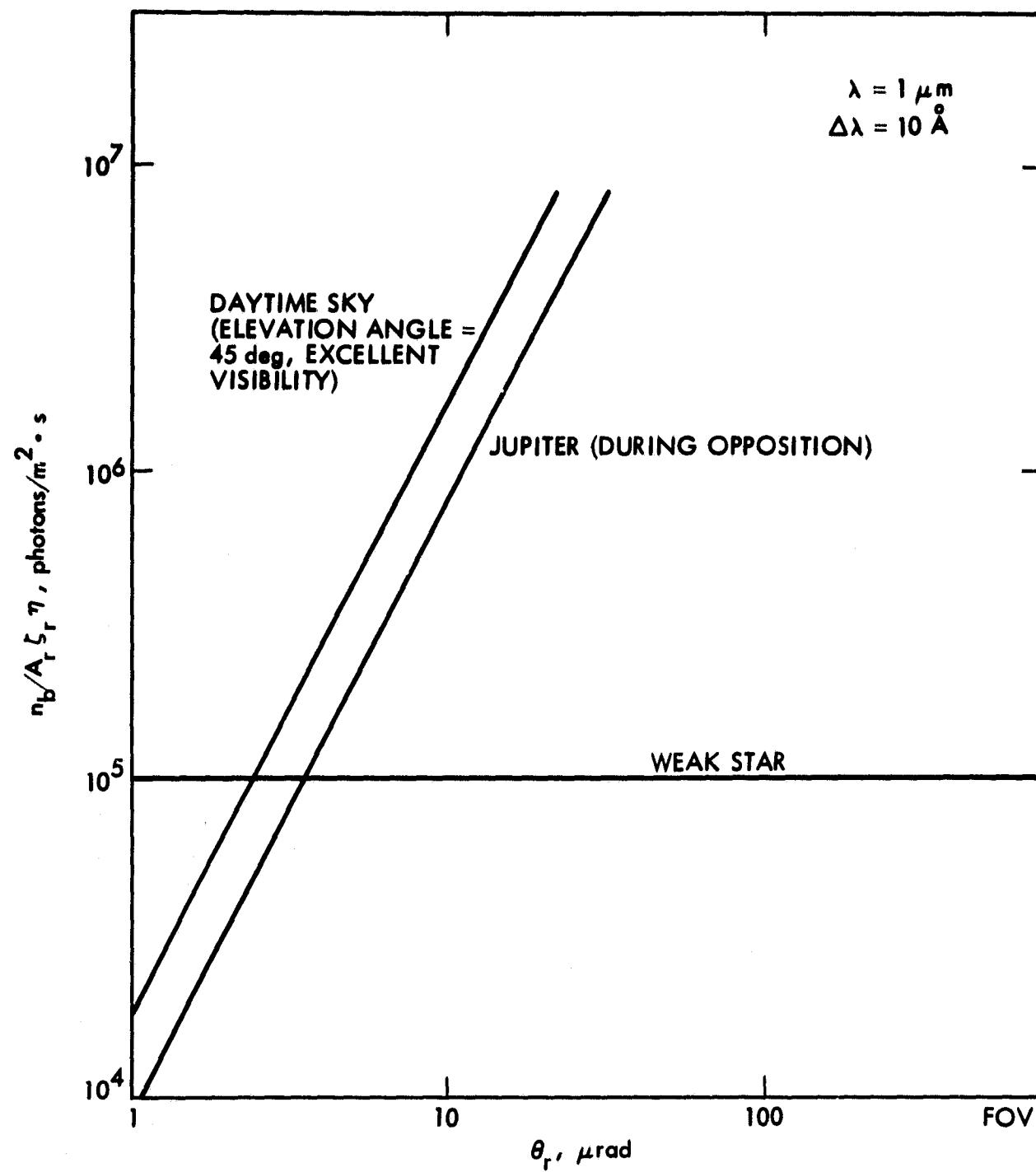
Figure B-1. Normalized Photon Rate as a Function of Receiver FOV for a Terrestrial Receiver
