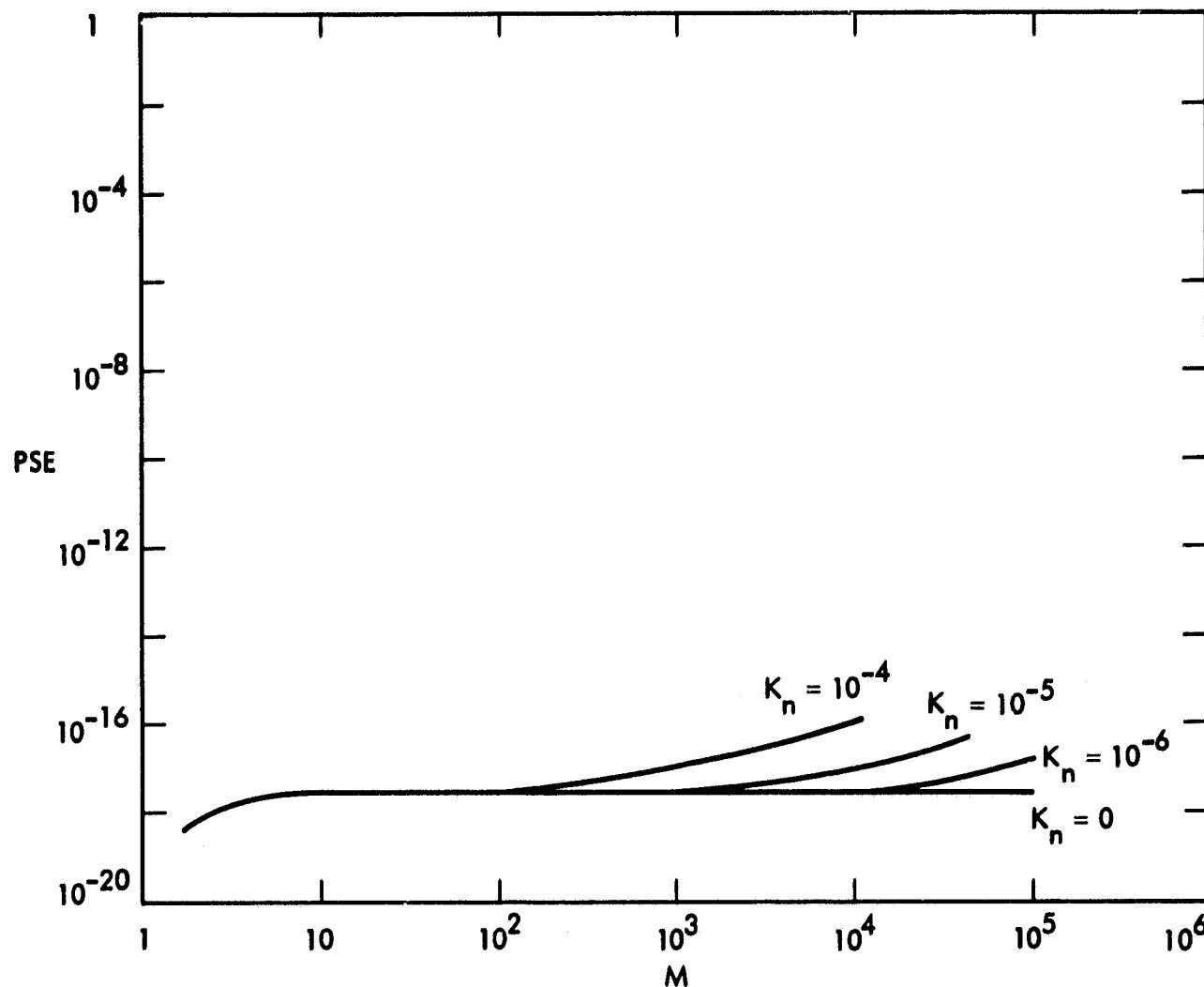
Figure 7-4. PPM Symbol Error Probability as a Function of M and
