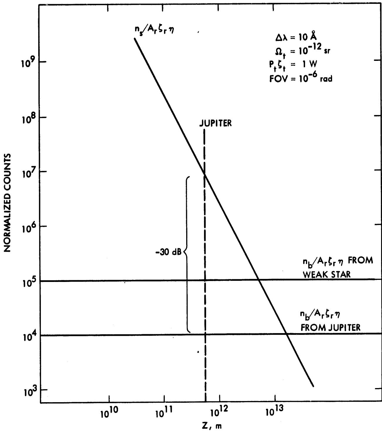
Figure B-3. Comparison of Signal and Background Counts, FOV = 1  $\mu\text{rad}$
