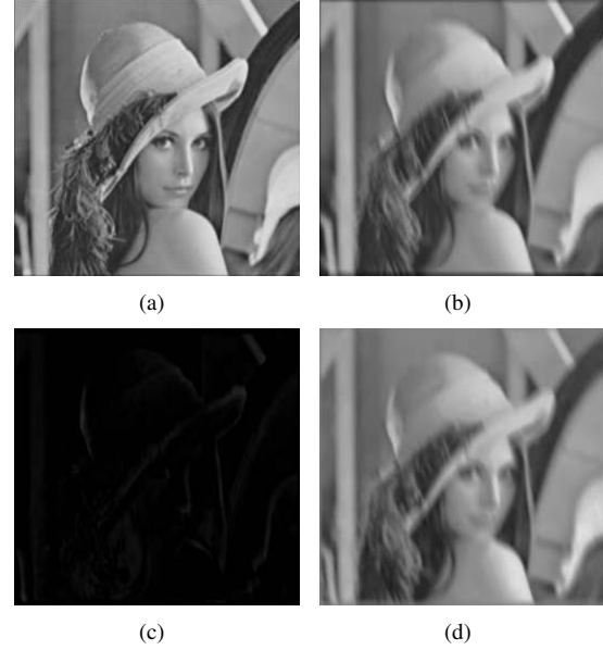
Figure 9. Result of spatially varying blurring. (a) a sharp image. (b) synthetic blurry image from projective geometry. (d) result of our optical computing system (c) residual between (b) and (d).
