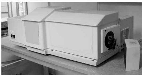
Figure 31: Lambda-900 spectrophotometer. The sample holder for reflectance measurements is shown to the right. Photo: M. Brogren.
