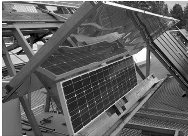
Figure 23: Testing of a crystalline silicon module with a planar over edge reflector of anodised aluminium, at Vattenfall Utveckling AB. Photo: M. Brogren.
