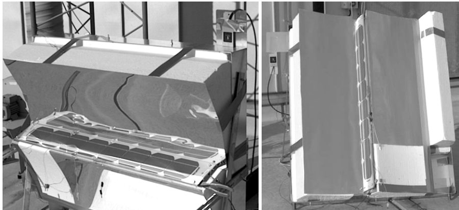
Figure 39: Experimental setup for outdoor measurements of short-circuit current as a function of solar height and current-voltage characteristics at different solar heights (left). Close to the equinox, the system was rotated 90° and tilted 30° backwards for simulation of all solar heights during a single day (right). Photo: M. Brogren.
