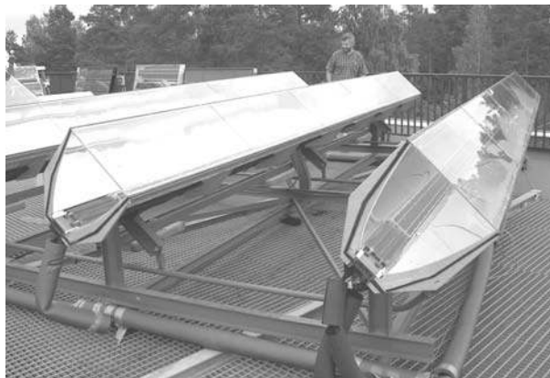
Figure 65: 4X concentrating photovoltaic-thermal system, which is installed in Älvkarleby (60.5°N, 17.4°E), Sweden. Photo: M. Brogren.
