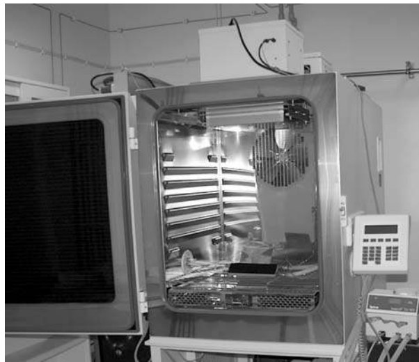
Figure 36: The climatic test chamber. Photo: K. Gelin.
