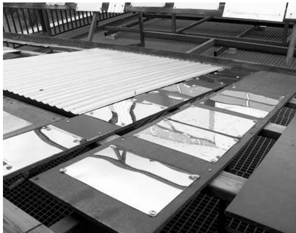
Figure 38: Reflector samples mounted for outdoor ageing at Vattenfall Utveckling AB's test facility in Älvkarleby. Photo: M. Brogren.
