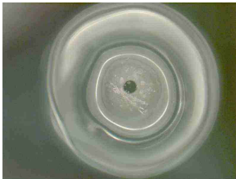
Figure 3.59. Micrograph of diaphragm and ferrule laser bonding (top view).
