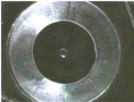
Figure 3.14. Ferrule and diaphragm bonded with ring.
