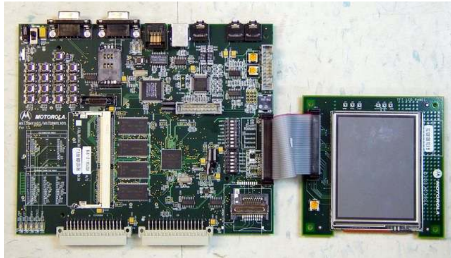
Figure 9.37. Motorola i.MX1 ADS.
