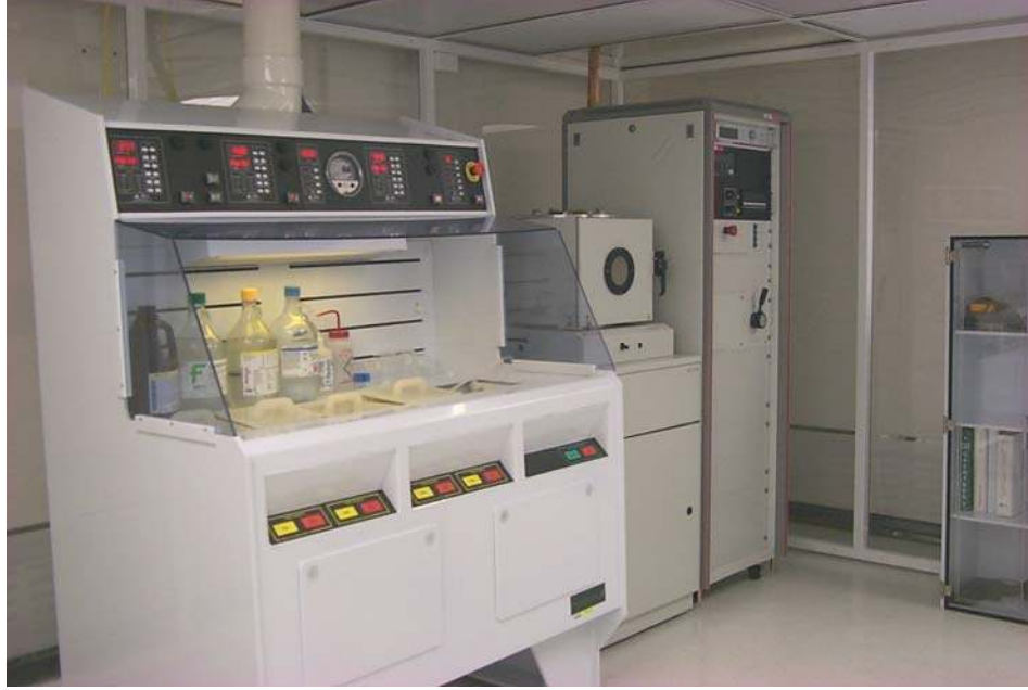
Figure 3.9. Bold Technology wet processing station (left) and Edwards AUTO 500 Sputtering System (right).
