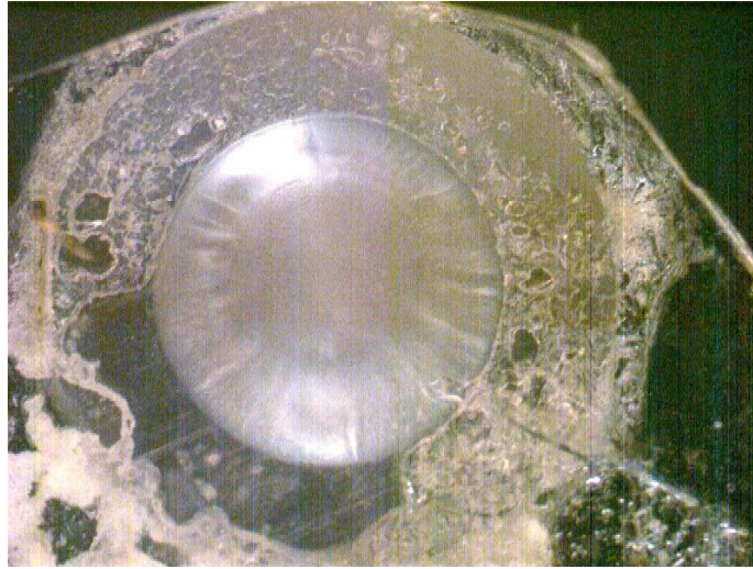
Figure 3.44. Interface of a wafer bonded with a ferrule bonded using the mechanism of hydroxide-catalysis bonding.
