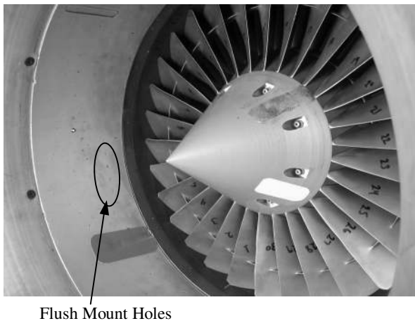
Fig. 12. Engine pressure sensor installation.
