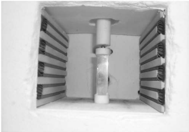
Fig. 9 Cubic zirconia block in high-temperature furnace for mechanical pressure testing.
