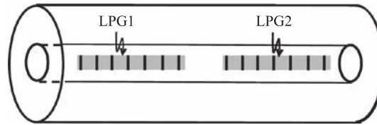
Figure 20: Schematic of a MZI formed with a pair of LPGs separated by a certain distance. LPG 1 induces partial coupling of power from the core mode to a cladding mode, which after propagating as a cladding mode re-couples back to the core mode after interacting with the second LPG. These two sets of beams taking different paths, when recombine after the second LPG form interference pattern that is characteristic of a MZI.
