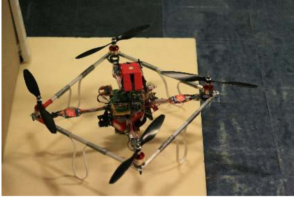
Fig. 2. Four rotor helicopter with cameras
