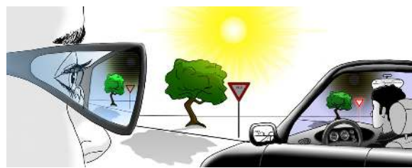
Figure 1: A conceptual illustration of our approach. A light modulation display locally filters a real-world scene to enhance the visual performance of a human observer, in this case by reducing the contrast of the sun and boosting the saturation of the traffic sign for a driver. Our approach would apply to see-through scenarios such as car windshields and eye glasses as depicted, as well as to binoculars, visors, and similar devices.
