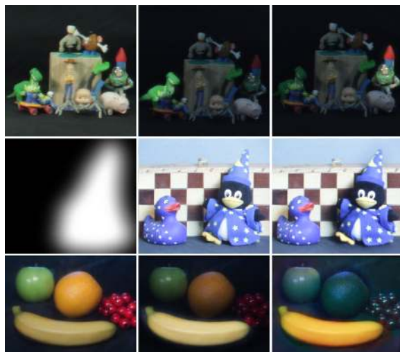
Figure 8: Example of object highlighting. Top row: object highlighting by darkening all but the region of interest. Middle row: more subtle direction of attention (right) by selectively sharpening some regions (left) of the image (center). Bottom row: highlighting by brightness (center) and color (right) manipulations using our second setup.
