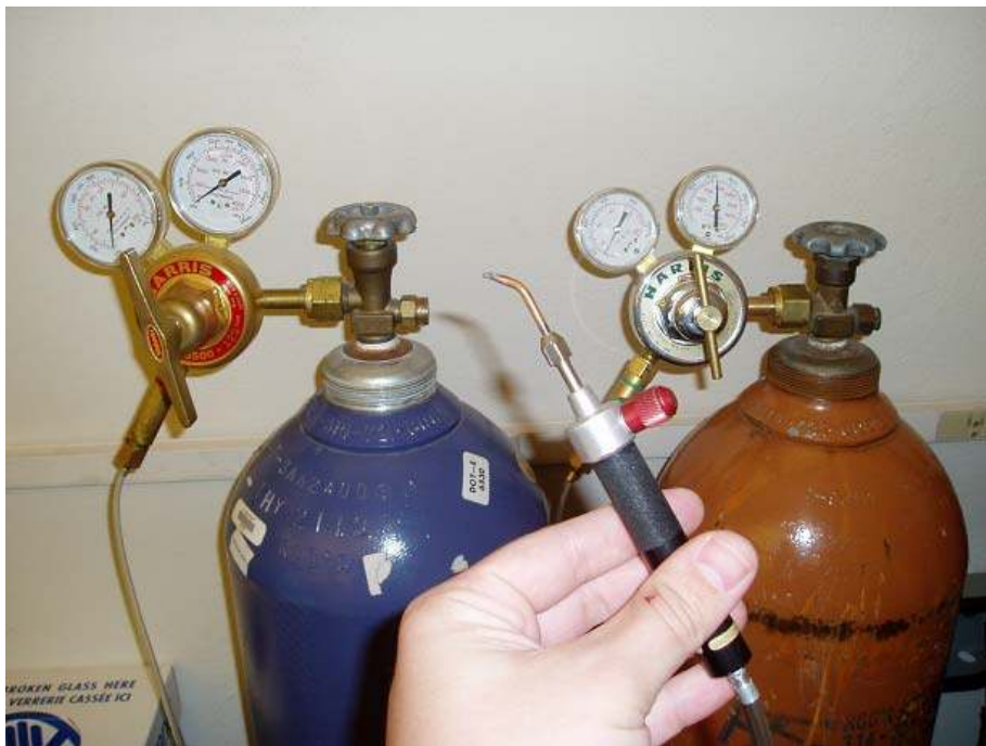
Figure A.7: H 2 /O 2 cylinders and torch
