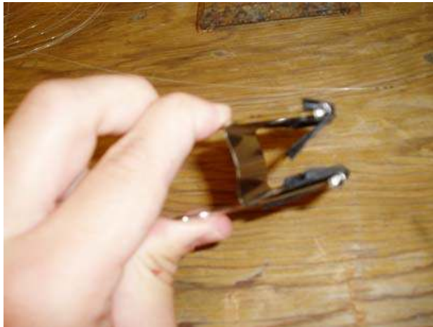
Figure A.9: Weight used to pull the fiber optic cable taut
