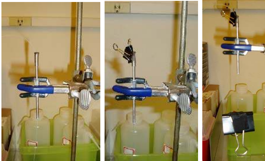
Figure A.8: Stand for suspending the fiber optic cable for flame cutting
