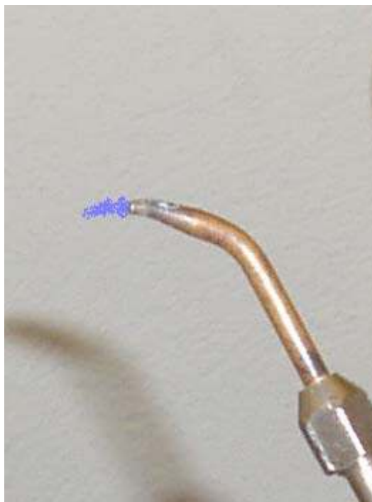
Figure A.14: Size and shape of intense H 2 /O 2 flame
