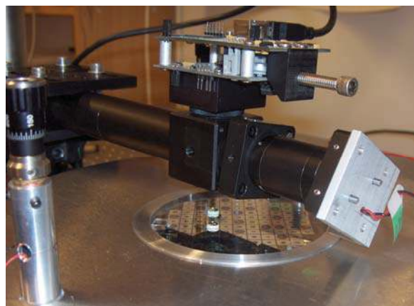
Figure 11 Experimental setup LCI, left: sketch of the wafer based Mirau configuration, right: photo of the setup.
