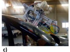
Fig. 3 Measurement of gap/flush in assembly of automotive vehicles: setup developed by Tran and Ha [34]. a Camera-laser module (high-resolution camera and a multi-line laser-based sensor), **b** view of the
