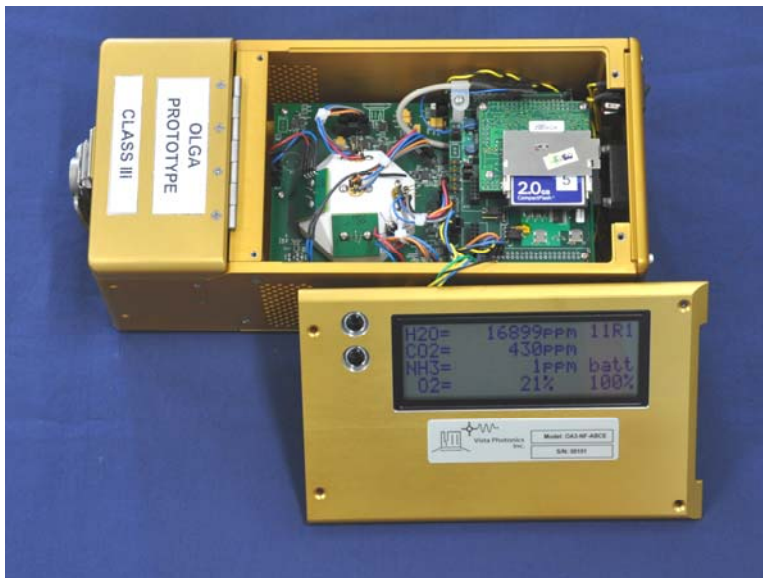
Figure 4. OLGA version 3.0. The custom FPGA board plugs directly into the main analog electronics board that controls the lasers. The sensor updates the significantly larger LCD and writes to file every 2.5 s, faster than the 7 s of earlier versions.
