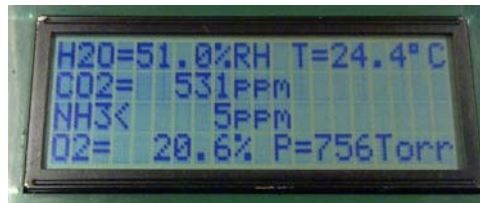
Figure 6. Multi-Gas Monitor display. Flight prototype instrument displays four measured gas concentrations, temperature and pressure. Display updates once per second.
