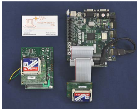
Figure 3. Custom and COTS FPGA. Reduction of the electronics footprint was enabled by using the custom FPGA board in the left of the photograph.
