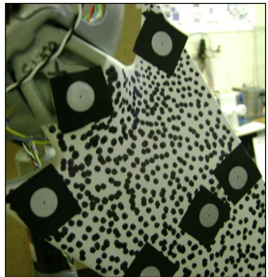
Figure 1. Example of prepared measurement surfaces: speckling for DIC and circular retroreflective targets used for dynamic photogrammetry.
