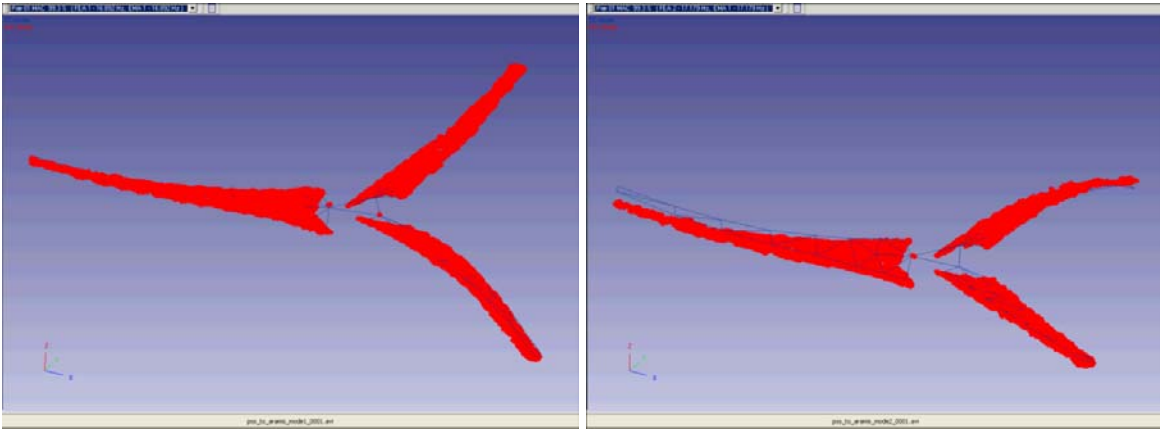
Figure 3. MIMO and FNMT DIC shapes for (a) mode 1 – 16.8 Hz; (b) mode 2 – 17.2 Hz.
