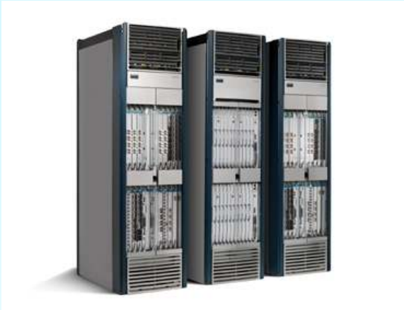
Cisco CRS-1 with 1000 ports, 250 ms buffering per port
