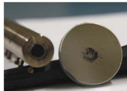
Figure 13. Soot deposits on optical surfaces.
