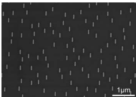
FIG. 1. SEM image showing the arrangement of a typical array of nanoparticles.
