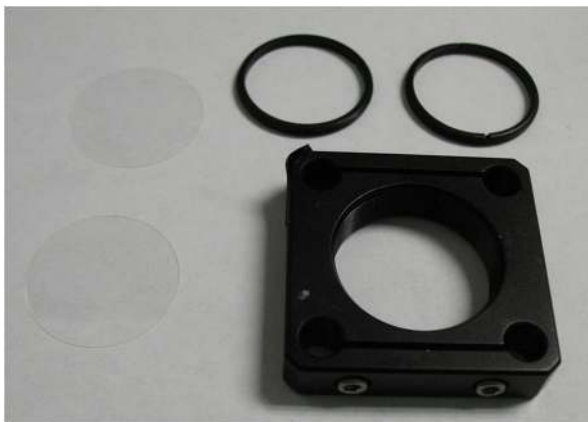
Fig. 1 Components of tissue holder, which is used to immobilize the tissue and keep the tissue thickness uniform during imaging. The tissue holder consists of a 30-mm threaded optic holder, two 25-mm circular glass slides, and two 30-mm threaded retaining rings used to evenly compress and sandwich the glass slides together against the tissue.
