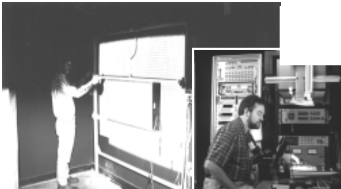
Fig. 1. Large (left) and small (right) scale solar simulators forevaluating PV performance in the laboratory.
