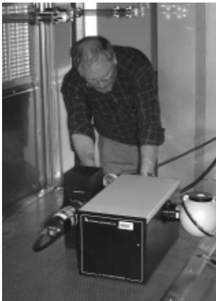
Fig 3. Scanning grating monochromator with integrating sphere input optic.
