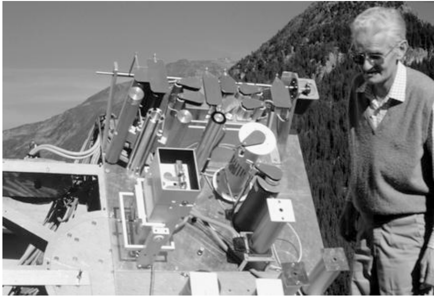
Fig. 7. World Standard Group of absolute cavity radiometers, the mean of which establish the World Radiometric Reference), maintained at the World Meteorological Organization World Radiation Centre in Davos Switzerland.
