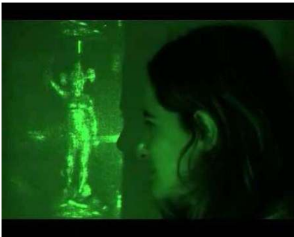
Fig. 2. (Color online) (Media 1) A spectator observing the acquired hologram SLM optical reconstructions, projected on a screen. The size of the image reconstructed at visible wavelength was about 30 cm, comparable to the original object size.
